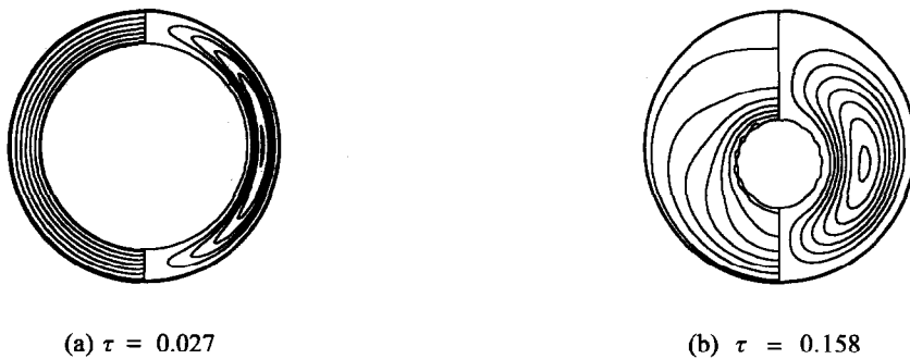
Fig. 7. The isotherms (left) and velocity contour (right) at Ra = 1.0 \times 10^4 , Ste = 0.045 and Sc = 0.004 .
